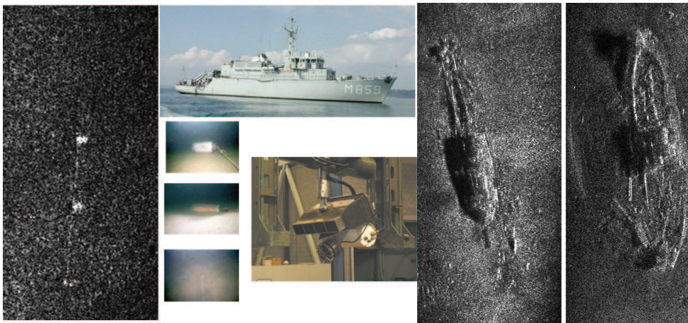
Fig. 4. Low frequency SAS images. On the left, SAS image of three cylinders. Downwards : proud cylinder, half buried cylinder, buried cylinder. In the middle : pictures of the supporting ship, the sonar and the three cylinders. On the right, SAS images of two wrecks in the bay of Brest.
