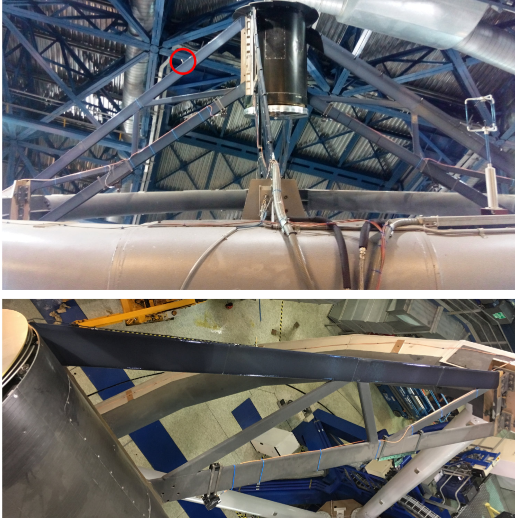
Figure 12. Top: View of the top ring, secondary mirror, and spiders after the coating. The 3-axis supersonic anemometer of the top ring is also visible on the right and one of the two thermocouples used in the temperature analysis is shown with a red circle. Bottom: View of one of the four spiders while one of the two parallel 20cm-beams was coated and the other not.
