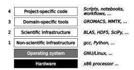
Fig. 1. A typical scientific software stack
