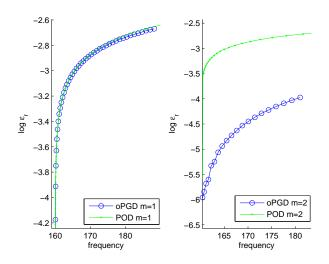
**FIGURE 8**. RELATIVE ERROR  $\varepsilon_r$  FROM THE REFERENCE SOLUTION FOR POD AND oPGD FOR m = 1, 2 (MNL computation)
