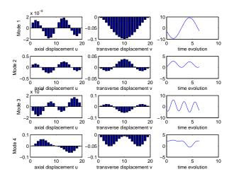
**FIGURE 4.** DECOMPOSITION OF THE SOLUTION COMPUTED BY oPGD FOR m=4 AT  $\frac{\omega}{2\pi}=180$  (shape have been normed for the purpose of comparison)
