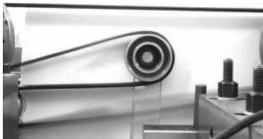
Fig. 2 Example of instability in slack belt span
