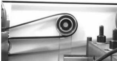
Fig. 2 Example of instability in slack belt span
