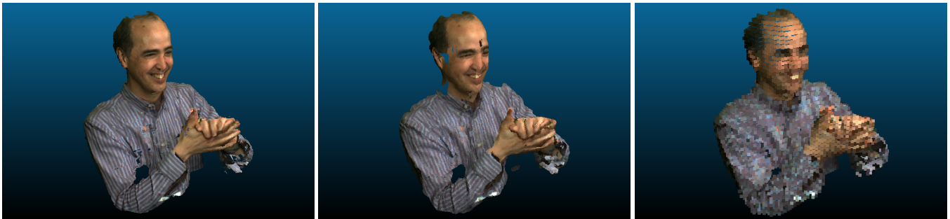
Fig. 4: Original point cloud (left), the compressed point cloud using the proposed method (middle) and the MPEG anchor (right). Colors are mapped using nearest neighbor matching. Our compressed point cloud was compressed using \lambda = 10^{-6} with a PSNR of 29.22 dB and 0.071 bpov. The anchor compressed point cloud was compressed using a depth 6 octree with a PSNR of 23.98 dB and 0.058 bpov. They respectively have 370,798; 1,302,027; and 5,963 points.
