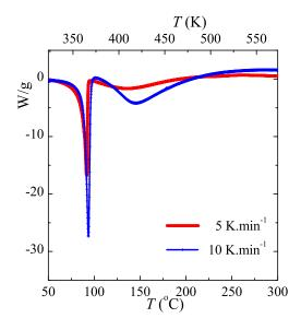
Figure 9: DSC curves showing the energy versus temperature for different heating rates. The deposit is about 500 layers of colloidal silica (1.16  $\mu m$ ) imbibed in 10  $\mu$ L of heptane.
