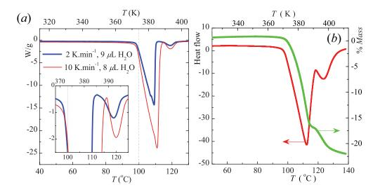
Figure 8: (a) DSC curves of 1.16  $\mu$ m deposits showing the energy versus the temperature for different scanning rates. The inset is a magnification of the second peaks. (b) TGA curves showing the energy and weight loss versus the temperature.
