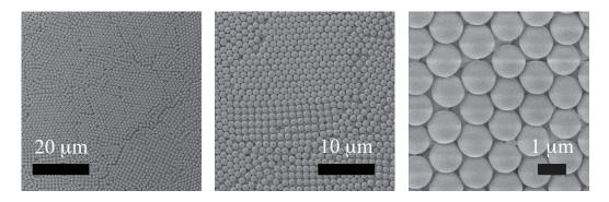
Figure 1: SEM images of an arrangement of silica micro-spheres of 1.16  $\mu$ m in diameter
