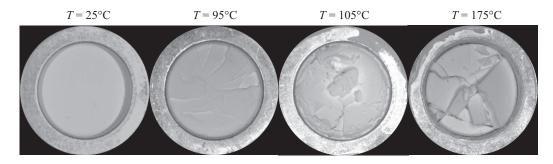
Figure 6: Micrographs of cracked patterns after drying of silica crystal of deposits of about 500 layers of 1.16  $\mu$ m diameter micro-spheres. The deposits were prepared in aluminium crucibles of 5 mm inner diameter.
