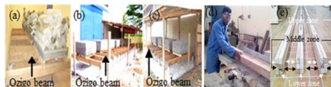
Figure 2. a) Air-conditioned environment. b) Unsheltered outdoor environment. c) Sheltered outdoor environment d) Alignment of the beam. (e) Test specimens for the characterization of spatial variability.
