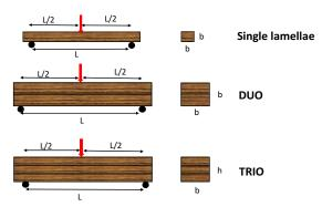
Figure 2. Different types of the tested beams on three-point bending.
