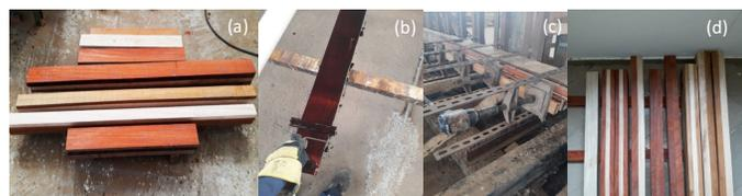
Figure 1. Gluing process: (a) boards planed, (b) grammage, (c) Presse, (d) GST beams.
