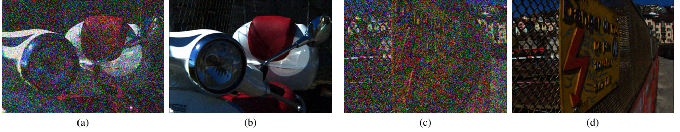
Fig. 1: 4D tensor driven diffusion is able to denoise highly damaged light fields. Center views for Vespa and DangerDeMort from the EPFL dataset. (a,c) With Additive Gaussian noise ( \sigma = \frac{100}{255} , PSNR= 8.13 dB); (b,d) After denoising giving global PSNR on all subapertures of 29.31 dB (b) and 28.50 dB (d).
