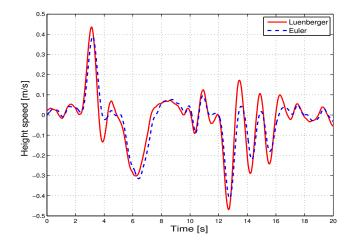
**Figure 6.** Altitude speed estimation comparison. The Luenberger estimator shows a faster response and smaller attenuations compared to the filtered Euler derivative.
