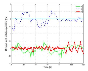
Figure 12. Drone's position relative to the targey. The UAV is able to follow the objective and keep a constant distance of 2m in front of it.
