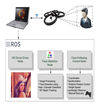
**Figure 2.** Overall system description. The drone communicates wirelessly with a ground station composed by a computer running ROS. Three main ROS nodes are executed in the ground station; the drone's driver, the face detection using OpenCV and the control node.
