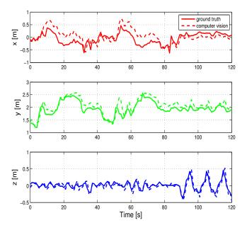
**Figure 9.** Relative position estimated by the computer vision algorithm (dashed line) vs ground truth (solid line). The proposed algorithm proves to be consistent with respect to the ground truth, but presents a small error.
