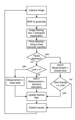
Figure 3. Flowchart of the image processing algorithm.
