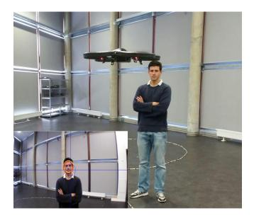
**Figure 1.** Detection and tracking of a mibile object using an UAV, application to following a human user. The UAV is able to autonomously follow the target of interest, keeping a constant distance with it.
