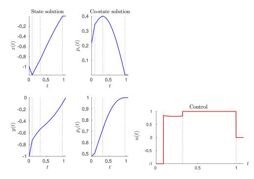
Figure 5: Time evolution of an extremal for the problem (28) of reaching the origin in minimal time starting from (x(0), y(0)) = (-1, -1).
