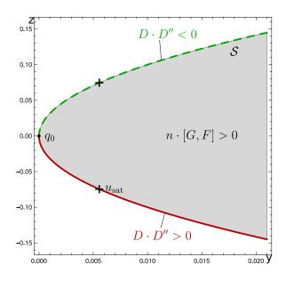
Figure 18: Stratification of N for the system (37). Green dotted line: elliptic, red line: hyperbolic, crosses: saturating values of the singular control.
