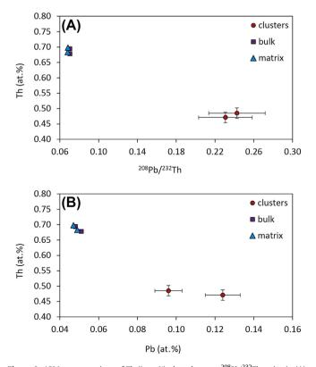
**Figure 6.** APM concentrations of Th (in at.%) plotted versus  $^{208}$ Pb/ $^{232}$ Th ratios in (A), and versus Pb concentrations (in at.%) in (B) from both APM tips prepared in D1-domain (Table 2). Clusters (in red) are enriched in Pb and depleted in Th compared to the bulk (purple) and the matrix (blue).
