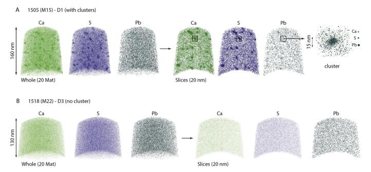
**Figure 4.** Reconstructed three-dimensional atom probe microscopy (APM) images of Ca, S and total Pb distribution in sample M15 (1505) prepared from cluster-rich-D1 domains (A) and sample M22 (1518) from cluser-free-D3 domains (B). Each sphere represents one atom. Slices (20 nm thick) from these 3D-images are also presented and a close up of one cluster in (A).
