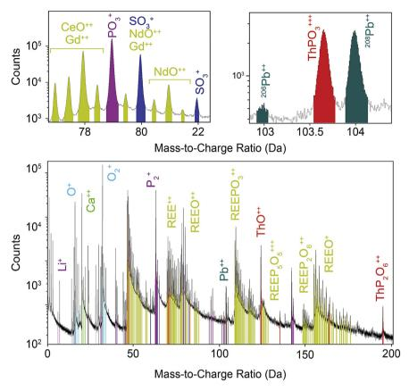
**Figure 3.** Atom probe mass spectrum. Peaks are color-coded by atomic or molecular species. Details of the mass spectrum showing the position of the SO<sup>+</sup><sub>3</sub>, CeO<sup>++</sup>, Gd<sup>++</sup>, NdO<sup>++</sup>, <sup>208</sup>Pb<sup>++</sup>, <sup>208</sup>Pb<sup>++</sup> and ThPO<sub>3</sub> + Peaks.
