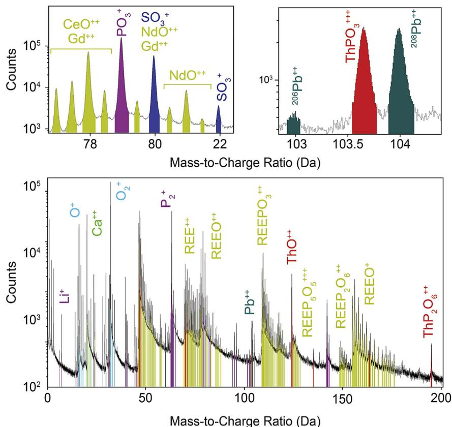
**Figure 3.** Atom probe mass spectrum. Peaks are color-coded by atomic or molecular species. Details of the mass spectrum showing the position of the  $\text{SO}_3^+$ ,  $\text{CeO}^{++}$ ,  $\text{Gd}^{++}$ ,  $\text{NdO}^{++}$ ,  $^{206}\text{Pb}^{++}$ ,  $^{208}\text{Pb}^{++}$  and  $\text{ThPO}_3^{+++}$  peaks.
