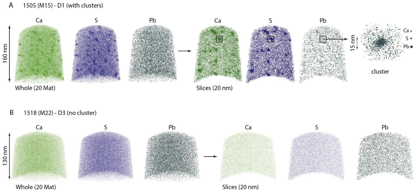
**Figure 4.** Reconstructed three-dimensional atom probe microscopy (APM) images of Ca, S and total Pb distribution in sample M15 (1505) prepared from cluster-rich-D1 domains (A) and sample M22 (1518) from cluster-free-D3 domains (B). Each sphere represents one atom. Slices (20 nm thick) from these 3D-images are also presented and a close up of one cluster in (A).
