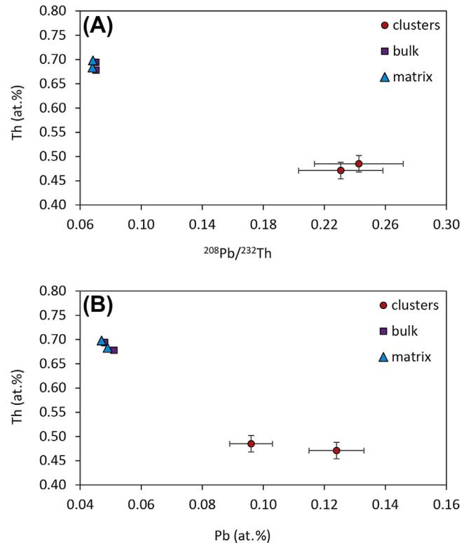
**Figure 6.** APM concentrations of Th (in at.%) plotted versus  $^{208}\text{Pb}/^{232}\text{Th}$  ratios in (A), and versus Pb concentrations (in at.%) in (B) from both APM tips prepared in D1-domain (Table 2). Clusters (in red) are enriched in Pb and depleted in Th compared to the bulk (purple) and the matrix (blue).
