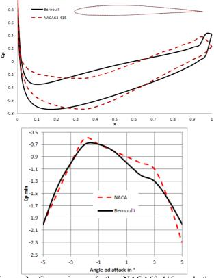
Figure 3. Comparison of the NACA63-415 and the equivalent Bernoulli profile. Top: profiles and *Cp* curves at  $0^{\circ}$  angle of attack. Botton: Variation of the *Cpmin* against the angle of attack.
