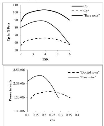
Figure 5. Comparison between the rotor in the symmetrical section duct and a bare rotor with a same cross section area. The Cp (top) computed using the rotor diameter gives the advantage to the ducted rotor but using the total area as a reference,  $Cp^*$ , produces much lower values than the bare rotor. The output power (bottom) as a function of the rotational velocity clearly indicates that the ducted rotor with a same cross section area than the bare rotor will produce far less energy.
