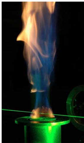
Figure 2: Photograph of the turbulent Bluff-Body flame
