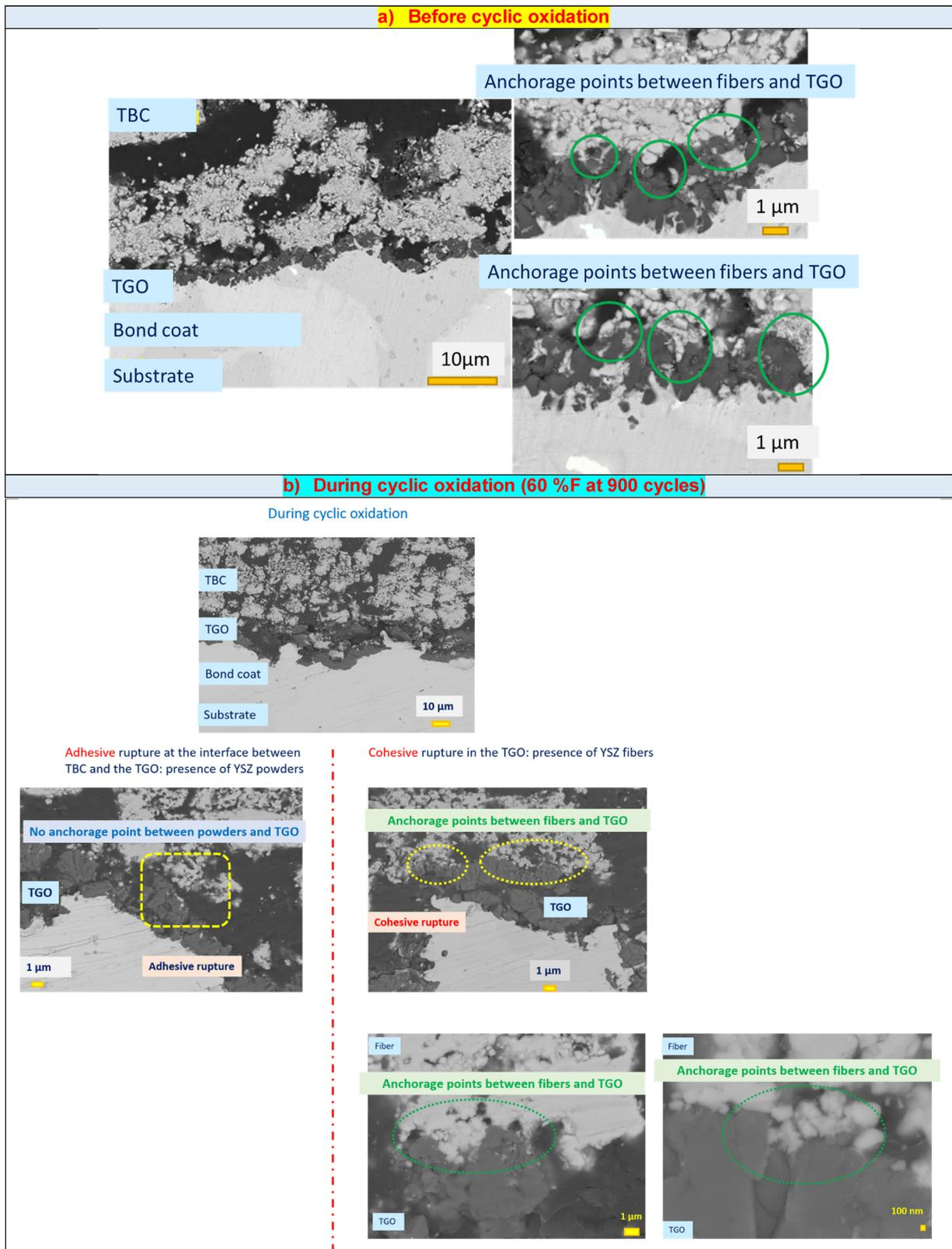
**Fig. 11.** SEM-FEG micrographs of the sections of TBCs to observe anchorage points between fibers and TGO layer: (a) before cyclic oxidation; (b) during cyclic oxidation (TBC with 60 %F at 900 cycles).
