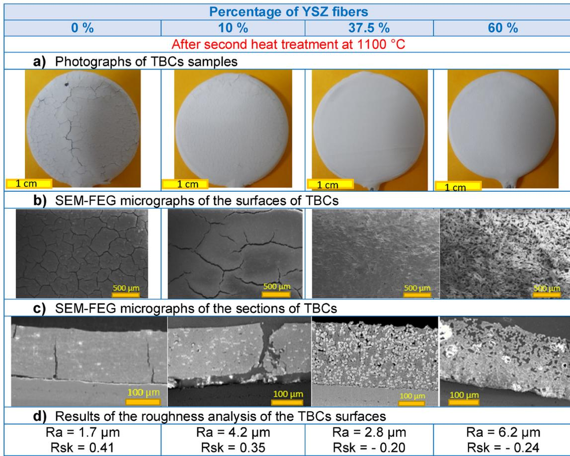
**Fig. 3.** Analysis of the surface and the cross-section of sol-gel TBCs versus the YSZ fibers percentage in the range 0% and 60% after heat treatment at 1100 °C: (a) photographs of TBCs samples; (b) SEM-FEG micrographs of the surfaces of TBCs; (c) SEM-FEG micrographs of the cross-sections of TBCs; (d) Results of the roughness analysis of the TBCs surfaces.
