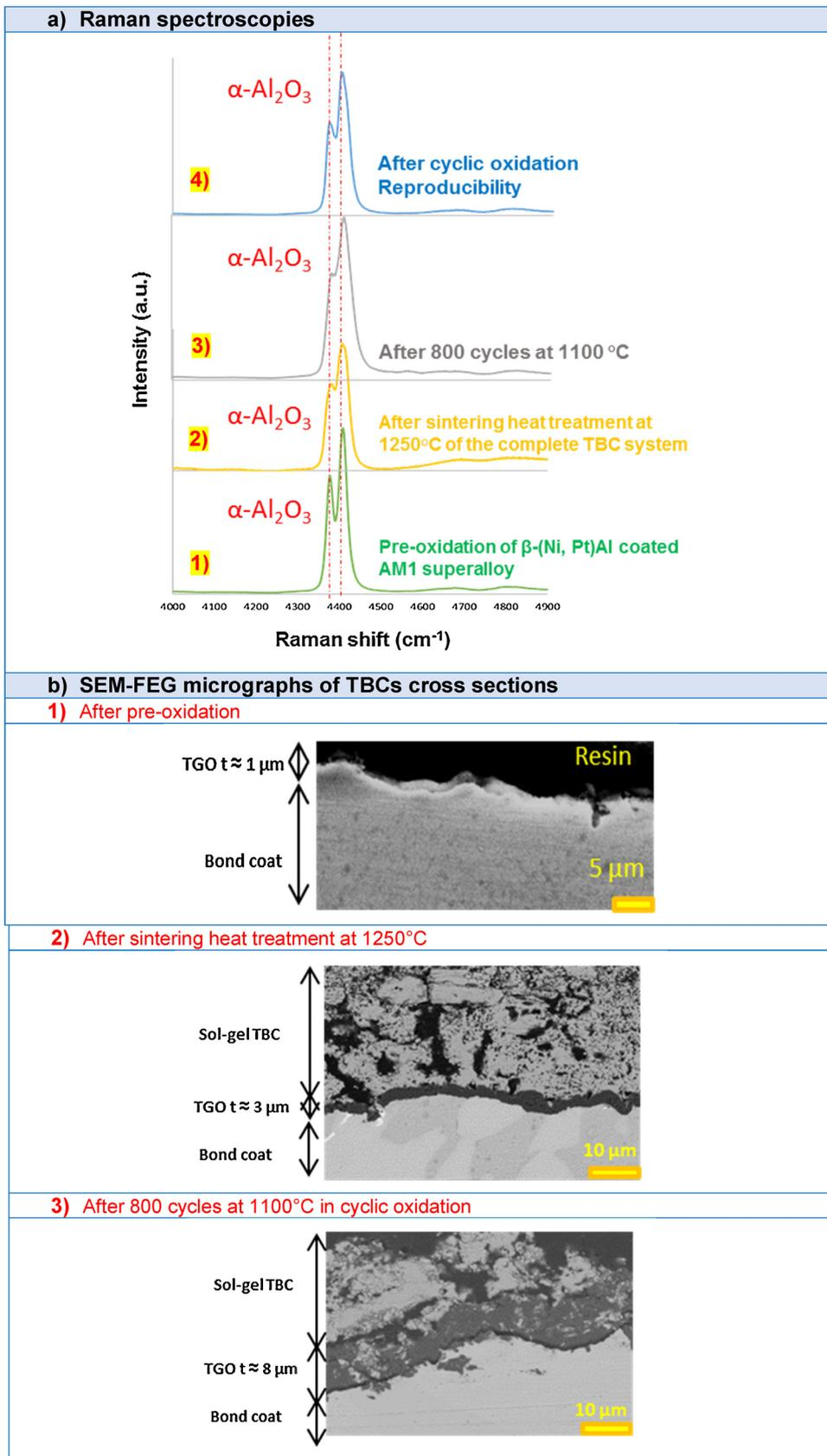
**Fig. 10.** Analysis of  $\alpha\text{-Al}_2\text{O}_3$  phase of TGO: (a) Raman spectroscopies of the TGO after: (1) pre-oxidation, (2) sintering heat treatment at 1250 °C; (3) 800 cycles at 1100 °C; (4) reproducibility check after cyclic oxidation (more than 1000 cycles) ; (b) SEM-FEG micrographs of TBCs cross sections observed after: (1) pre-oxidation, (2) sintering heat treatment at 1250 °C; (3) 800 cycles at 1100 °C.
