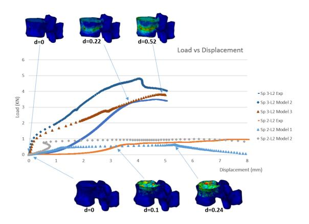
Figure 6: CT- Scan and F-E results for the six specimens: Damage localization zones when the ultimate experimental load is reached for the three models.
