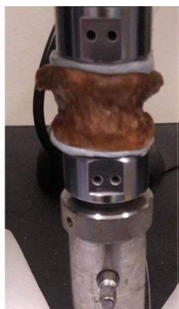
Figure 2 a : Lumbar vertebra before failure. The resin is placed at the top and the bottom of the vertebral body.
