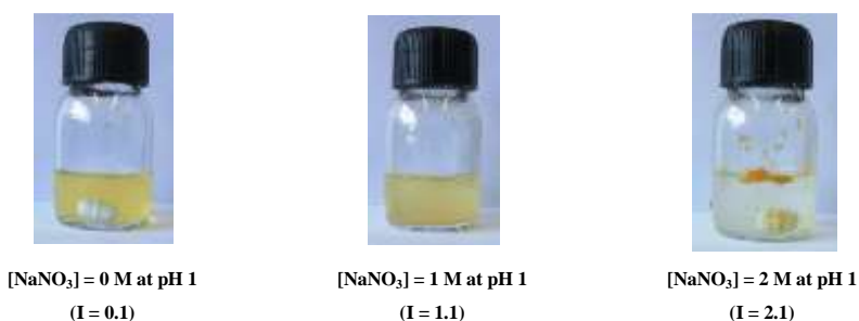
Fig. 7 Solutions of hPCPAAm6C obtained for various concentrations of \text{NaNO}_3 , for C_{hP(\text{CPAAm6C})} = 5 \text{ g.L}^{-1} and \text{pH} = 1 .
