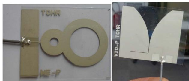
Fig. 1. View of a coaxial interconnection directly soldered to the PCB (courtesy of Technicolor Connected Home Company)
