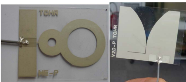
Fig. 1. View of a coaxial interconnection directly soldered to the PCB (courtesy of Technicolor Connected Home Company)
