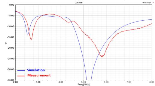
Fig. 8 - S<sub>11</sub> measured and simulated dual-band Wi-Fi dipole antenna
