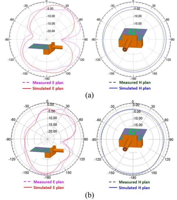
Fig. 5 E-Plane and H-Plane radiation patterns of dual-band Wi-Fi monopole antenna at: (a) 2.4 GHz and (b) 5.5 GHz
