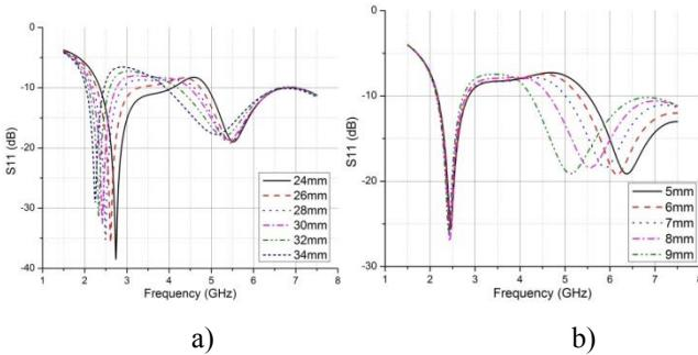
Fig. 3. Effects of changing L3 and L6 on the 2.4 GHz and 5.5 GHz frequencies
