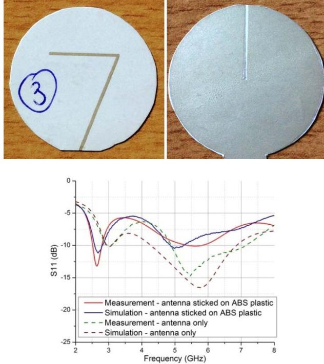
Figure 7: Prototype and return loss of a modified ultra-wideband dipole
