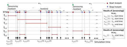
Fig. 4. System-level approach for the simulation of run-time mapping strategies through the dynamic control of the execution of tasks for different use-cases.
