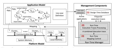
Fig. 1. System models with application, platform and management components descriptions.
