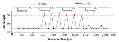
**Fig. 6.** Evolution of simulated  $A_1$  latency, captured for four different use-cases. Results are given for the LASP strategy [13].
