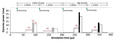
Fig. 7. Simulated dynamic power of  $A_1$  is captured with the advancement of simulation time. Results are given for  $uc_1$  according to different platform configurations.
