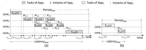
**Fig. 2.** A design-time prepared execution trace for the mapping of  $App_1$  (a) and  $App_2$  (b) on homogeneous cores, according to [13].
