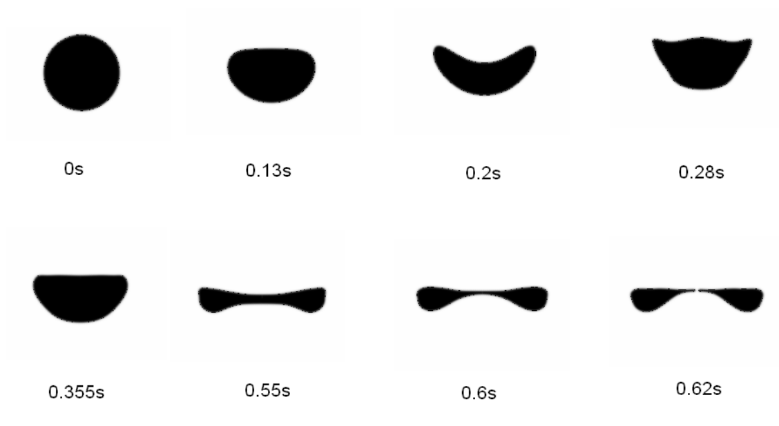
Figure 5: Deformation and thick rim shear breakup of an iron drop within a magma ocean. In this model, Re = 36.4 , We = 14.6 , R_\mu = 200 (simulation #30 in Table 2).
