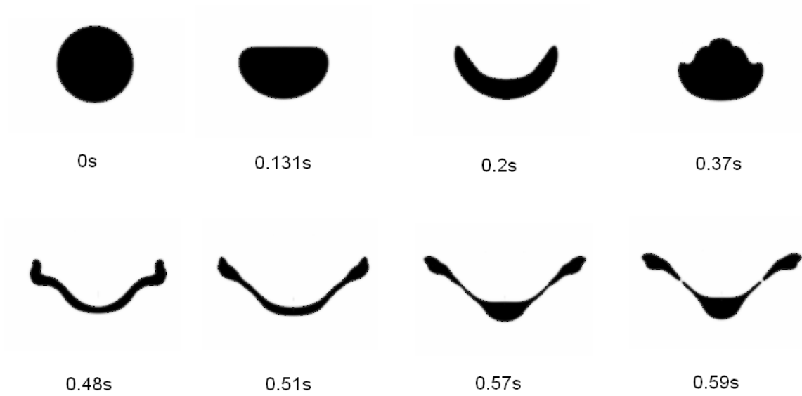
Figure 7: Deformation and rim shear breakup of an iron drop within a magma ocean. In this model, Re = 92.4 , We = 20.3 , R_\mu = 100 (simulation #22 in Table 2).
