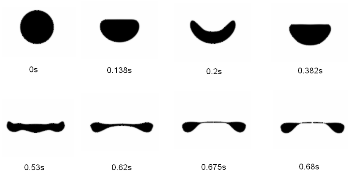
Figure 6: Deformation and thick rim bag breakup of an iron drop within a magma ocean. In this model, Re = 42.5 , We = 17.2 , R_\mu = 200 (simulation #32 in Table 2).
