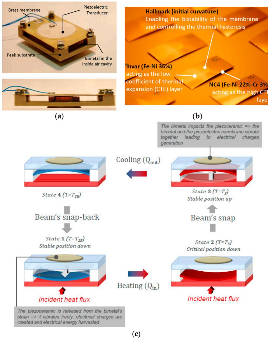
**Figure 1.** (a) Thermal energy harvester previously developed based on a piezoelectric membrane and a bimetallic strip in the inside air cavity; (b) Image of the precurved bimetal; (c) Working principle of the harvester and different states of the bimetal.
