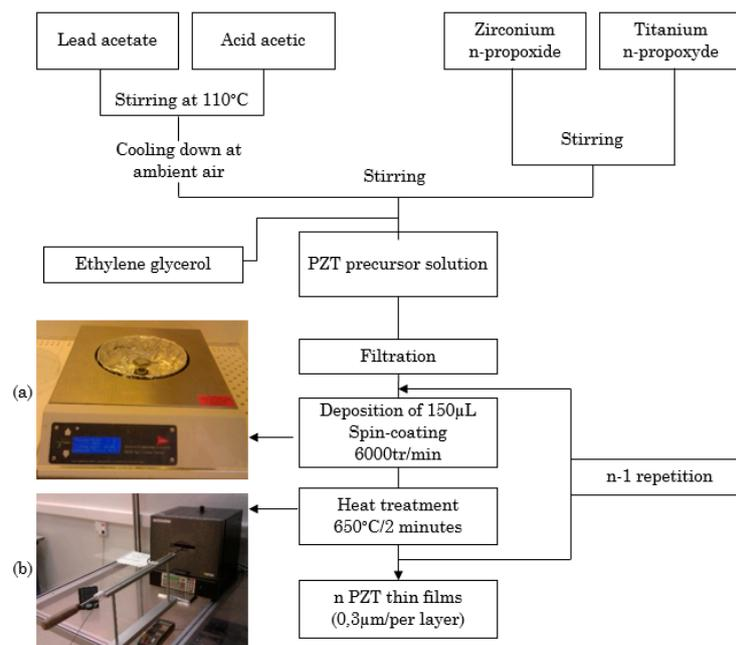
**Figure 3.** Deposition process of the PZT thin films (a) Spin coating equipment; (b) Oven used for the heat treatment of the thin films.
