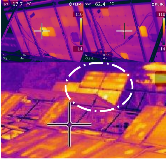
Fig. 11: Top : Two Infrared photographs of a module backsheet, with reflector augmentation taken 1 minute apart. A moving patchwork of hotspot cells is apparent. Bottom : view of multiple short-circuited modules. Only the modules highlighted with the white circle have reflector augmentation.
