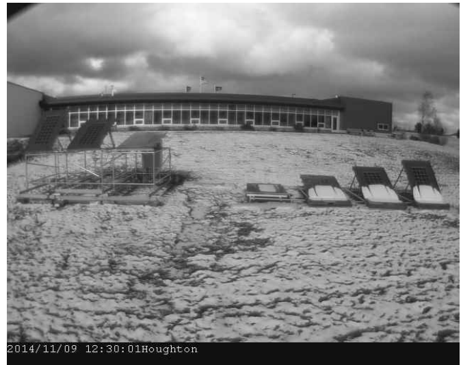
Fig. 1. 7-module snow test platform at the Keweenaw Research Center
