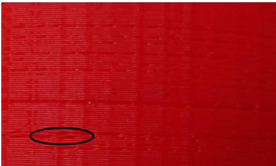
Figure 10. Under extrusion on exterior surface of 3D printed object (observable as dark lines).
