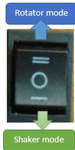
Fig. 11. Rotator mixer on one switch pole and shaker on another switch pole and center off.
