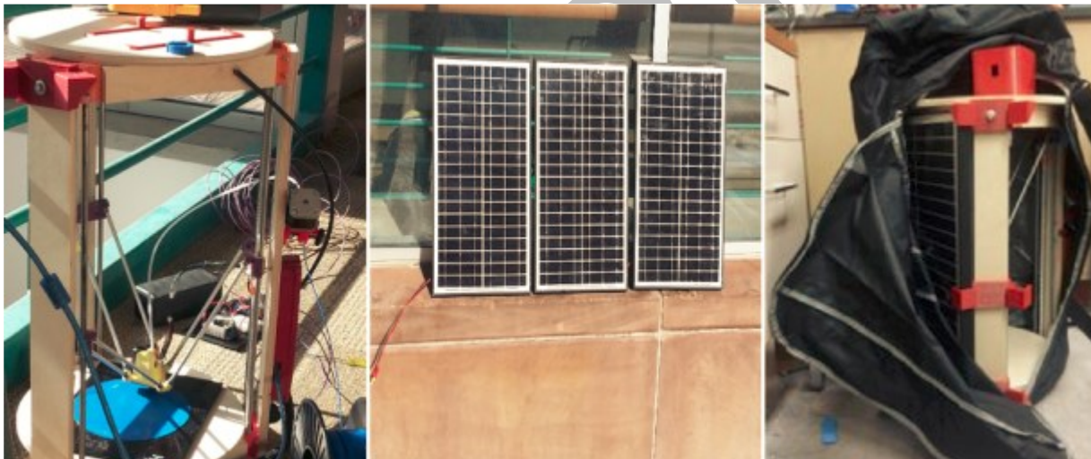
Fig. 1. Solar Powered MOST-delta 3-D printing, 3 x 12 V, 24 W solar panels, and printer with panel mounted in a duffel bag [25]. The PV modules are clipped to the frame of the RepRap for shipping.
