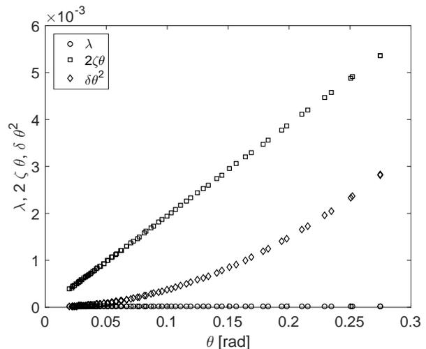
**Fig. 8** Relative importance of solid friction force ( $\lambda$ ), viscous force ( $\zeta$ ), and quadratic dissipative force ( $\delta$ ), as a function of the angle, for the experiment shown in Fig. 7.
