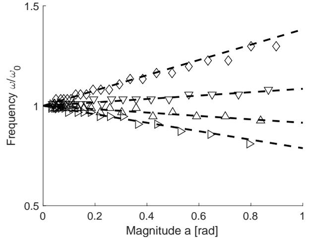
**Fig. 4** Evolution of frequency with amplitude for a pure quadratic elastic force  $\nu\theta^2\text{sgn}(\theta)$ . Symbols: numerical solution to Eq. (1) with initial conditions  $\theta(0) = 1$ ,  $\dot{\theta}(0) = 0$  (one value per half-period) with  $\zeta = 0.05$  and  $\nu=-0.5$  ( $\triangleright$ ),  $-0.2$  ( $\triangle$ ),  $0.2$  ( $\triangleright$ ),  $0.9$  ( $\diamond$ ). Broken lines: Eq. (9).
