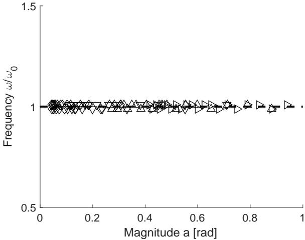
**Fig. 3** Evolution of frequency with amplitude for a pure quadratic dissipative force  $\delta\dot{\theta}^2\text{sgn}(\dot{\theta})/\omega_0^2$ . Symbols: numerical solution to Eq. (1) with initial conditions  $\theta(0) = 1$ ,  $\dot{\theta}(0) = 0$  (one value per half-period) with  $\delta=0.05$  ( $\triangleright$ ),  $0.1$  ( $\triangle$ ),  $0.3$  ( $\triangleright$ ) or  $0.8$  ( $\diamond$ ). Broken line: Eq. (9).
