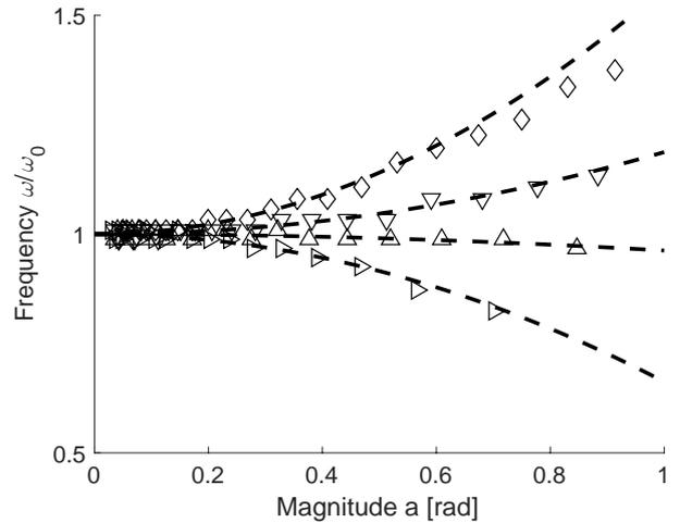
**Fig. 5** Evolution of frequency with amplitude for a pure cubic elastic force  $\epsilon\theta^3$ . Symbols: numerical solution to Eq. (1) with initial conditions  $\theta(0) = 1$ ,  $\dot{\theta}(0) = 0$  (one value per half-period) with  $\zeta = 0.05$  and  $\epsilon=-0.9$  ( $\triangleright$ ),  $-0.1$  ( $\triangle$ ),  $0.5$  ( $\triangleright$ ),  $1.5$  ( $\diamond$ ). Broken lines: Eq. (9).
