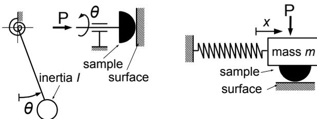
**Fig. 1** Left: principle of a torsional pendulum with a sphere/plane contact at the extremity of the rotation axis. Right: principle of a translational oscillator with a sphere in contact with a plane and attached to the moving mass.
