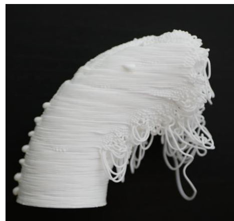
Fig. 14. Additive manufacturing with 2.5D path without support
