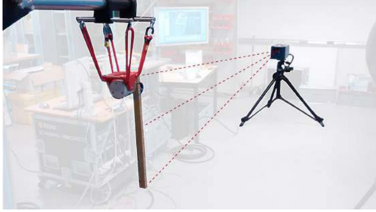
Figure 12: Experimental set-up for measuring the displacement field of the honeycomb sandwich beam. The structure is mounted on a shaker at location x_0 = 0.048 m, a scanning laser vibrometer estimates the transverse displacement field.
