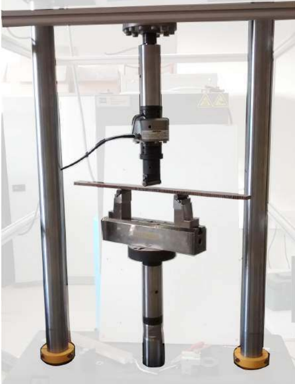
Figure 17: Experimental set-up for the three points flexural bending test. The beam is simply supported on two cylinders and a gradually increasing static load is assigned to the structure.
