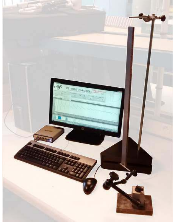
Figure 18: Experimental set-up for measuring the local displacement field of the honeycomb sandwich with free boundary conditions. A mini-hammer is impacting the beam at the location of a mini-accelerometer.
