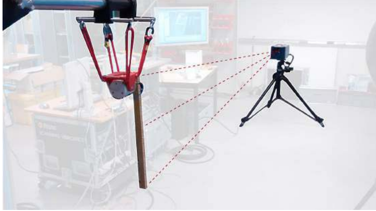
Figure 12: Experimental set-up for measuring the displacement field of the honeycomb sandwich beam. The structure is mounted on a shaker at location x_0 = 0.048 m, a scanning laser vibrometer estimates the transverse displacement field.
