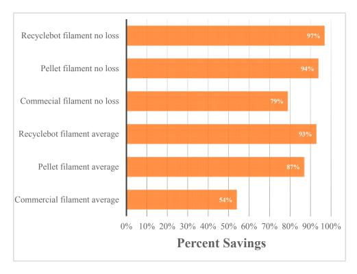
Figure 2. Bar chart showing the percent savings of printing designs with various filament types.
