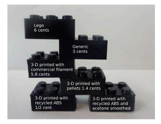
**Figure 4.** Photograph of  $2 \times 3$  toy bricks: Lego brick, Lego-compatible generic brick, 3D printed commercial ABS and 3D printed recycled acrylonitrile butadiene styrene (ABS) bothnatural and acetone smoothed with costs.
