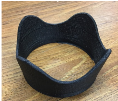
Figure 14. The camera hood printed a) with camera and b) with camera by the RepRap from recycled ABS filament.
