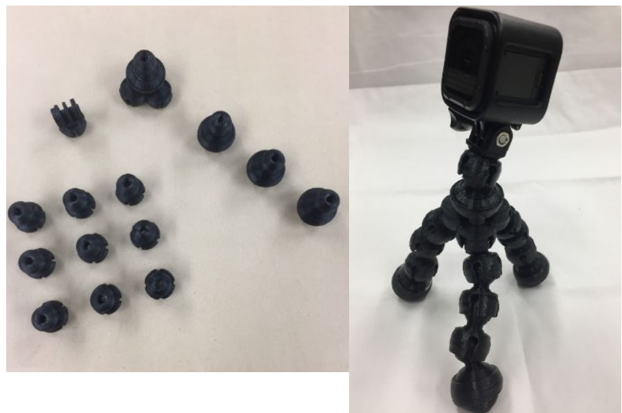
Figure 12. The camera bubble tripod printed a) components and b) assembled by the RepRap from recycled ABS filament.
