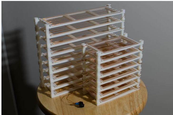
Figure 6. Comparing design options for the open-source slide dryer: 66-slide dryer behind a 30-slide dryer.
