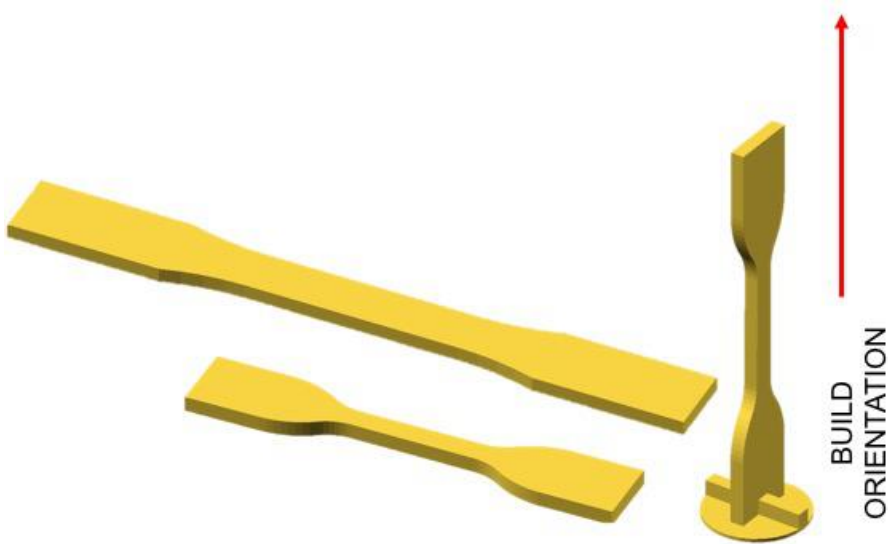
Fig. 1. Generated .stl files for the variants of ASTM D638-14 Type I vs. Type IV tensile bars.
