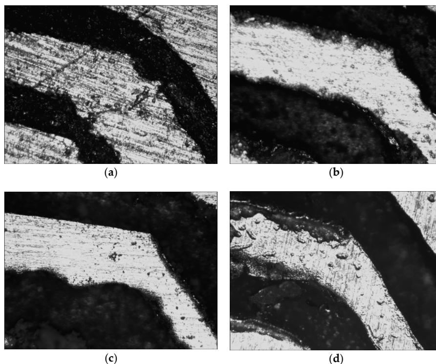
**Figure 10.** Top row from left to right: (a) Feed rate of 50 mm/min, plunge depth of 0.1 mm; (b) feed rate of 100 mm/min, plunge depth of 0.1 mm; (c) feed rate of 150 mm/min, plunge depth of 0.1 mm; and (d) feed rate of 50 mm/min, plunge depth of 0.2 mm.
