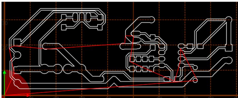
Figure 15. The rendered tool path in the XY-axis.
