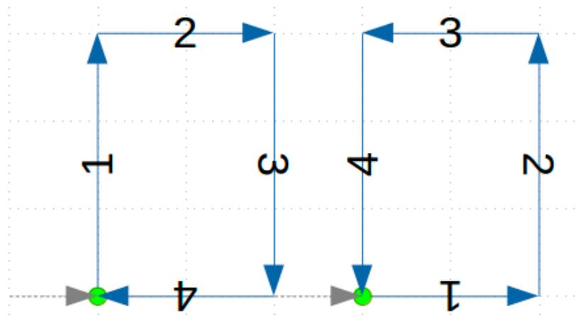
**Figure 8.** A test pattern to verify feature repeatability and backlash compensation effectiveness. Grey dashed arrows indicate that the mill is moving above the substrate. Green Circles indicate that the tool has plunged into the surface. Blue arrows indicate the path the mill is cutting into the copper.
