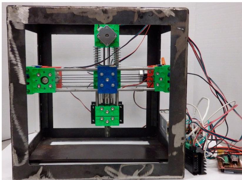
**Figure 9.** An image of the completed circuit mill.
