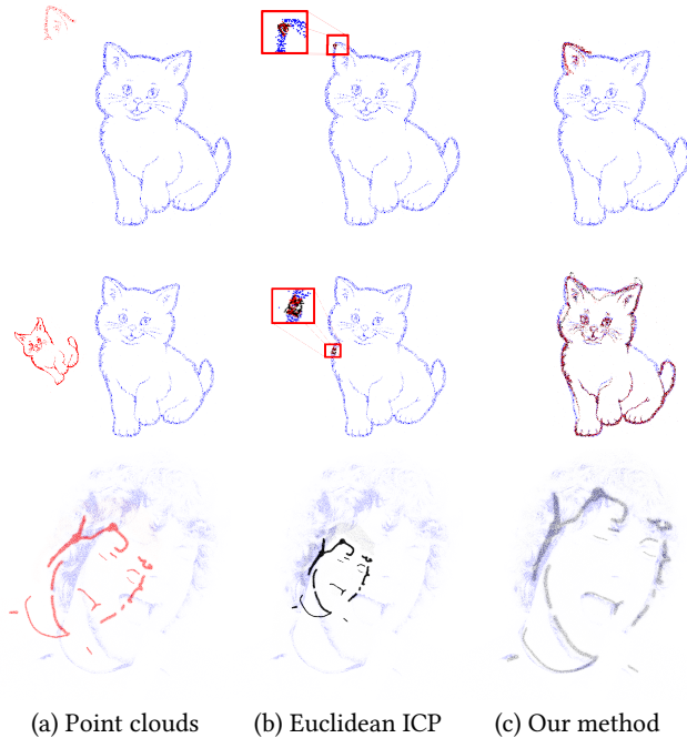
Fig. 7. We register the red to the blue point cloud in (a) using a similarity transform (translation, rotation and scaling). Samples on both point clouds are different. We used a classical Iterative Closest Point algorithm in (b) that uses nearest neighbors and our sliced partial transport matching in (c).
