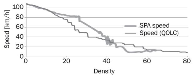
Figure 4 – Speed-density relationships obtained by both approaches
