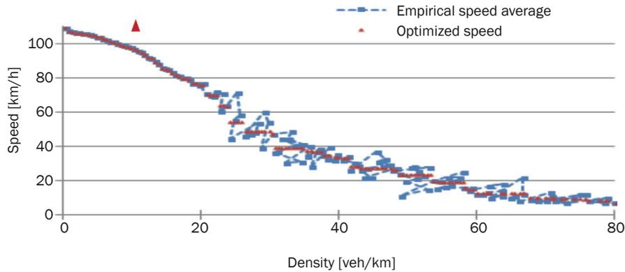
Figure 3 – Speed-density relationship with the QOLC approach
