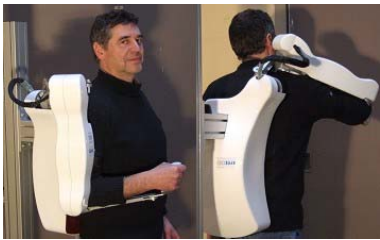
Fig. 5. ABLE 4 axis exoskeleton actuated by screw-and-cable actuators
