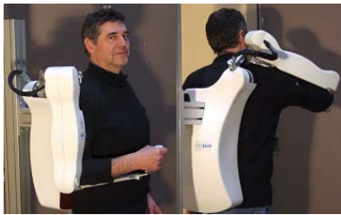
Fig. 5. ABLE 4 axis exoskeleton actuated by screw-and-cable actuators
