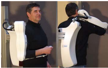
Fig. 5. ABLE 4 axis exoskeleton actuated by screw-and-cable actuators
