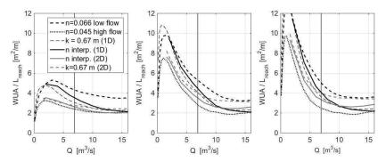
Figure 5 : WUA as a function of the discharge for the station 1 for different bed friction methods. Vertical line represents the annual averaged discharge. Left: adult, center: juvenile, right: alevin.
