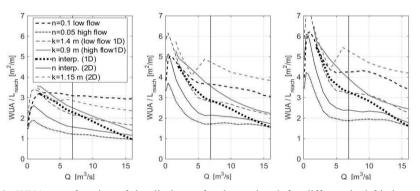
Figure 6 : WUA as a function of the discharge for the station 2 for different bed friction methods. Vertical line represents the annual averaged discharge Left: adult, center: juvenile, right: alevin.
