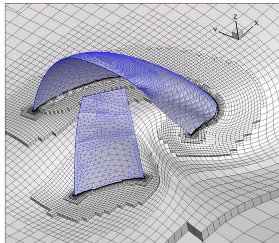
A new mesh deformation tool has also been developed to transmit the deformation of the sails to the fluid domain without having to rebuild a new grid from scratch. This method, based on the combination of an explicit advancing front method and smoothing is also
