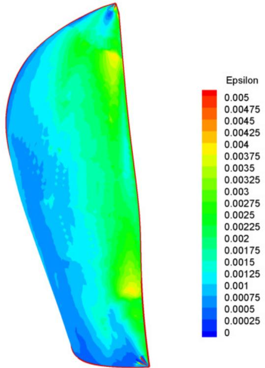
Sailmakers are also interested in other results such as the deformation of the cloth: *Figure 10* shows the mean deformation in the cloth. Maximum deformation of about 0.4% occurs near the luff, on both sides, near the reinforcements.
