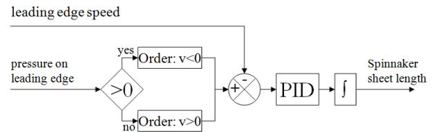
Some tests were needed to adjust PID parameters: too violent of a trimming algorithm work like a “pumping” trimmer, some waves appears and move on the sail. With too slow of an algorithm, the luff collapses hard, and the computation could stop, due to limits of the mesh deformations.
