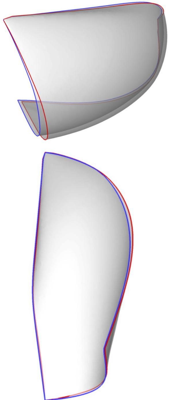
**Figure 8 : Comparison of the behavior of the luff for the two gennakers during 4 steps of the period.**
