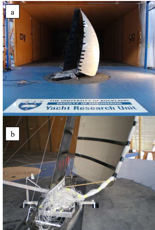
Figure 1: Photographs of the rigid spinnaker setup in the wind tunnel; (a) general view from downstream; (b) close-up view from behind the yacht model.
